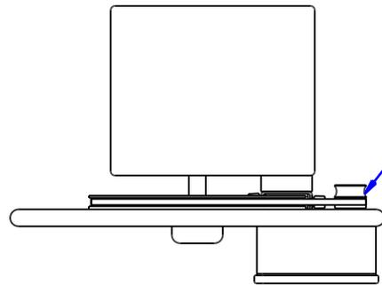
Clutch extends past edge of bulkhead to provide enough room to pull it out when disengaging autopilot. This is only necessary when the spoke-to-bulkhead distance is less than 2.25"
