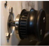
2. Make sure the ends of the two shear-pin screws are not bent, then remove the two screws from the back of the clutch. Remove the circlip, then remove the drive gear from the driveplate shaft.
