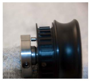
5. Lightly grease the motor shaft to prevent corrosion. Slide the clutch all the way onto the motor shaft and tighten the setscrew. Don't overtighten or gall the stainless threads. A bit of antiseize makes future removal easy. The setscrew may be torqued up to 62 in-lbs.
